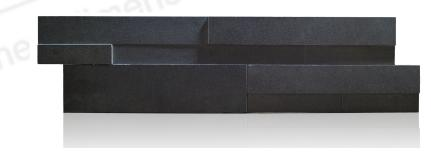
CORNER UNITS: 6" Tall by 24" Long with stepped interlocking ends, appx .94 sq ft in face coverage. Thickness varies between approx 1/2" to 5/8". Wraps 8" on one side and 16" on the other (see diagram).
